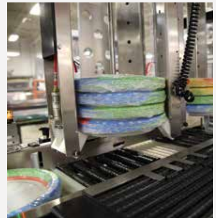
PLATE BUNDLE STACKING
