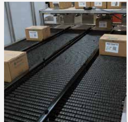
PACKAGES ENTER PALLET BUILD STATION
