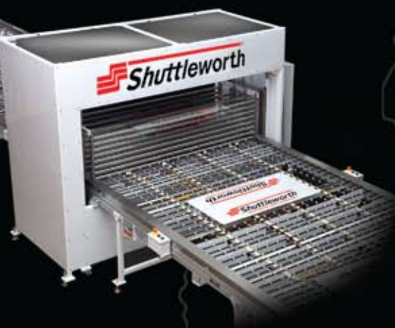
Zoned Accumulation Buffer
