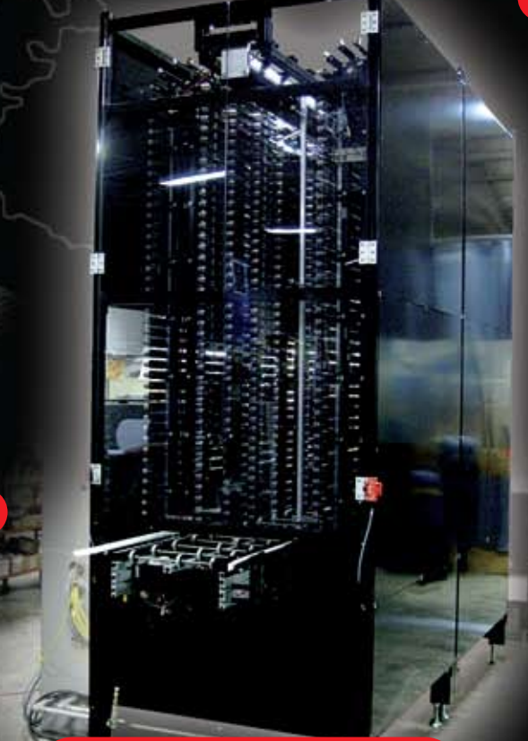
Inline LIFO/FIFO Buffer
